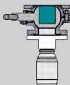
Filling the plug, defined volume
